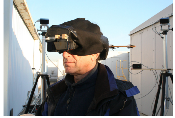
Figure 3: The HMD was retrofitted with thick black felt to block any unwanted ambient light to enter the eyes, which would have reduced the contrast of the overlay graphics. Three of the six cameras used for tracking can be seen as black boxes behind the participant.
