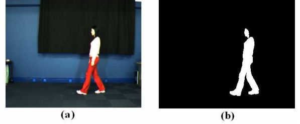
Figure 2. (a). Original image with person in the scene; (b). Binary image after subtracting background
