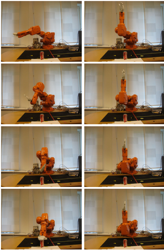
Fig. 4. A trajectory generated from random initial positions reaching for the same object
